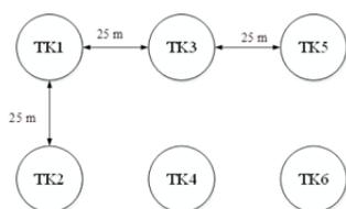
Figure 3: Layout of the gasoline tanks
