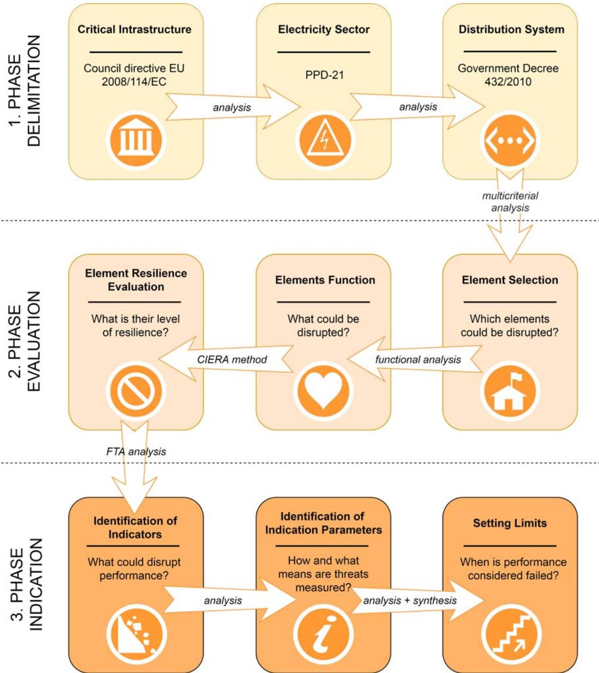
Figure 2: Predictive indication of performance failure in electricity critical infrastructure elements
