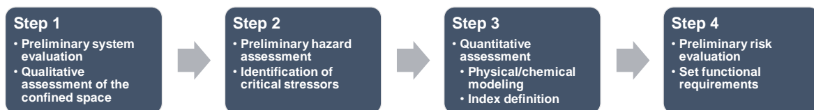
Figure 1: Flowchart of the methodology aimed at the quantitative assessment of confined space hazards.
