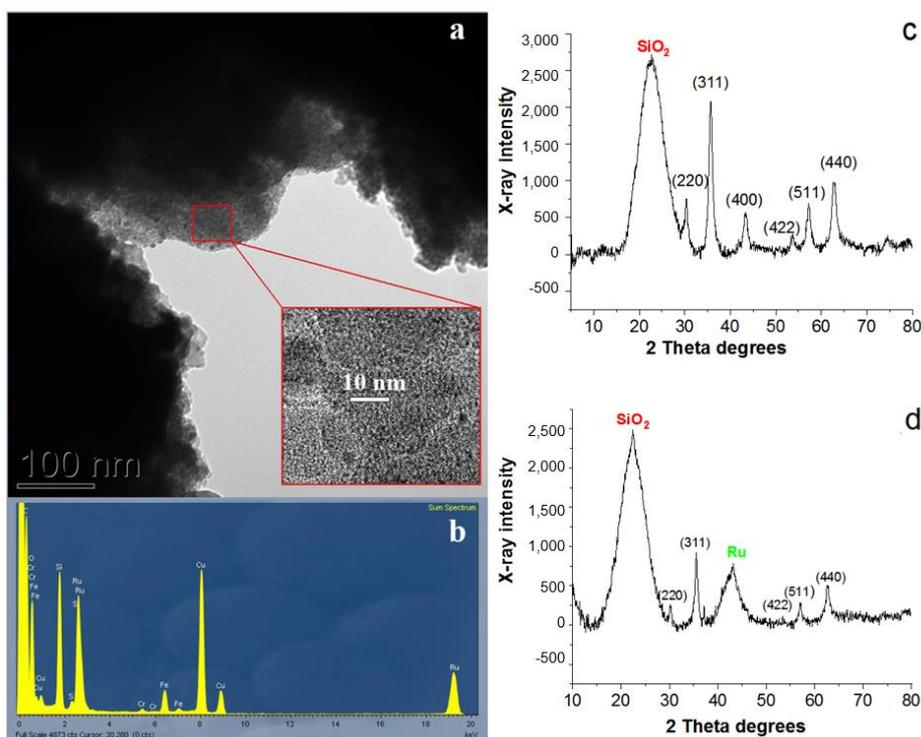
Figure 1: TEM image (a), EDS spectrum (b), and XRD pattern (d) of 5 % Ru-Fe<sub>3</sub>O<sub>4</sub>-SiO<sub>2</sub>. XRD pattern of Fe<sub>3</sub>O<sub>4</sub>-SiO<sub>2</sub> is shown in (c) for comparison. Inset in (a) shows the HRTEM image
