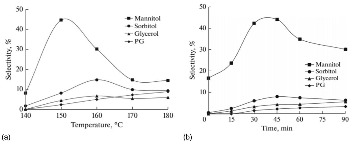
Figure 3: (a) Dependence of selectivity toward mannitol, sorbitol, glycerol, and PG on the process temperature (0.1167 mmol of Ru per gram of inulin; 0.3 g of inulin; 0.07 g of catalyst; 30 mL of H<sub>2</sub>O; H<sub>2</sub> 60 bar; 45 min) (b) Dependence of selectivity toward mannitol and secondary products on process time (0.1167 mmol of Ru per gram of inulin; 0.3 g of inulin; 0.07 g of catalyst; 30 mL of H<sub>2</sub>O; 150 °C; H<sub>2</sub> 60 bar)
