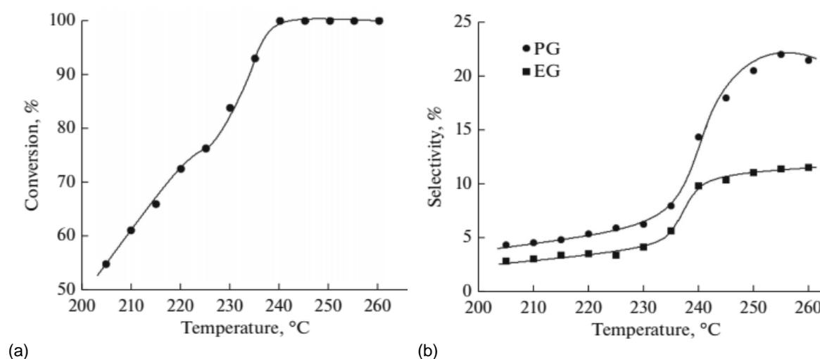
Figure 2: (a) Cellulose conversion as functions of the process temperature (0.1167 mmol of Ru per gram of cellulose; 0.3 g of cellulose; 0.07 g of catalyst; 30 mL of H<sub>2</sub>O; = 60 bar, 60 min) (b) EG and PG selectivity as functions of the process temperature (0.1167 mmol of Ru per gram of cellulose; 0.3 g of cellulose; 0.07 g of catalyst; 30 mL of H<sub>2</sub>O; = 60 bar, 60 min)
