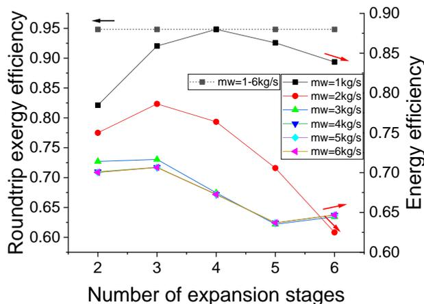
Figure 4: The energy efficiency, round-trip exergy efficiency under different water mass flow rate
