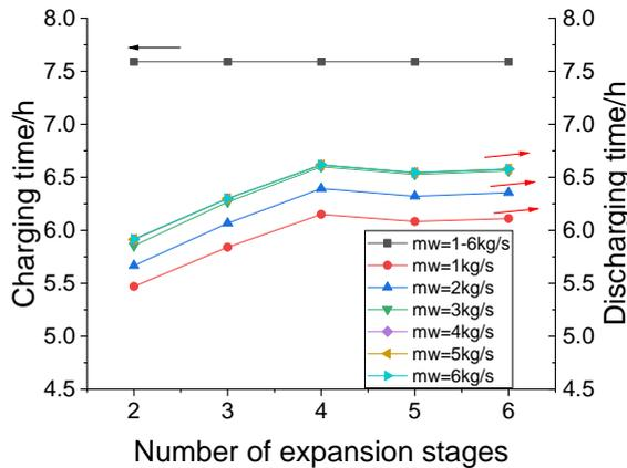
Figure 2: The trend of charging and discharging time
