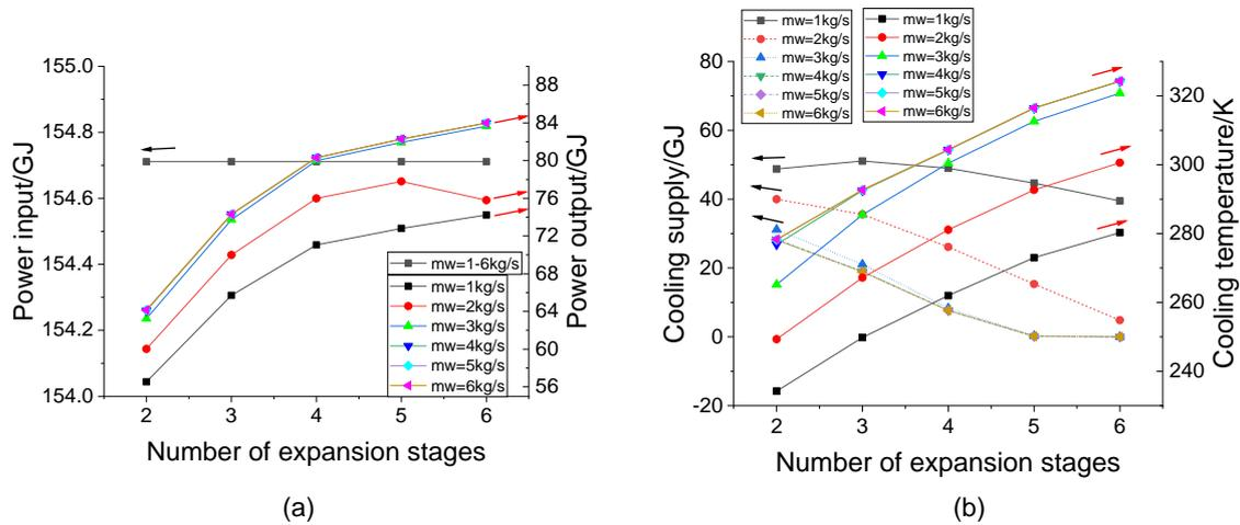
Figure 3: (a) The trend of power input and output (b) The trend of cooling supply and temperature
