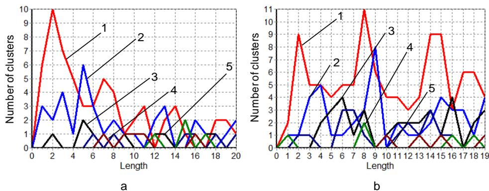
Figure 3: Dependences of the clusters number of different orders in the flow reactor ( $W=4$ ) on the longitudinal coordinate  $L$  ( $W=2$ ;  $T=24$ ), clusters orders: 1-first, 2-second, 3-third, 4-fourth, 5-five. A- DLA aggregation; B- mixed kinetics
