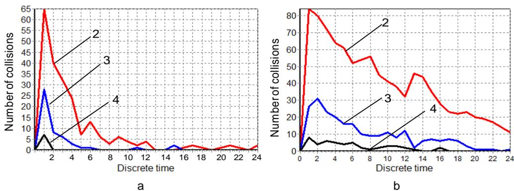
Figure 2: Time dependences of the collisions number of different orders in the batch reactor, collisions orders: 2-second, 3-third, 4-fourth. A- DLA aggregation; B- mixed kinetics
