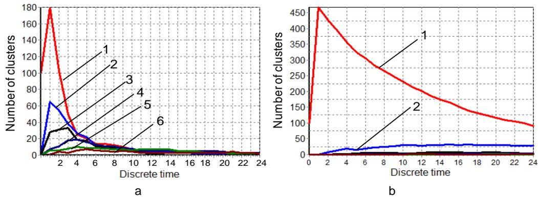
Figure 1: Time dependences of the clusters number of different orders in the batch reactor, clusters orders: 1- first, 2-second, 3-third, 4-fourth, 5-five, 6-six. A- DLA aggregation; B- mixed kinetics
