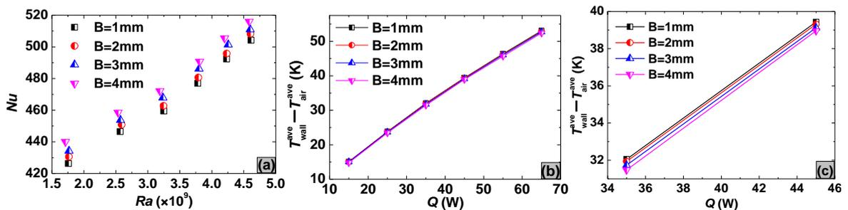
Figure 5: Effect of  $B$  on the air side heat transfer performance. (a)  $Nu$ , (b)  $T_{wall}^{ave} - T_{air}^{ave}$ , (c) Partial enlargement of b
