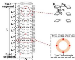
Figure 2: Schematic of finned tube structure and temperature measuring point arrangement
