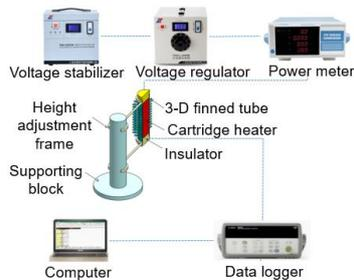
Figure 1: Schematic of the experimental system
