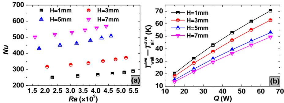
Figure 4: Effect of  $H$  on the air side heat transfer performance. (a)  $Nu$ , (b)  $T_{wall}^{ave} - T_{air}^{ave}$
