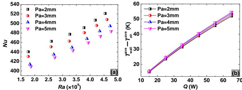
Figure 6: Effect of  $Pa$  on the air side heat transfer performance. (a)  $Nu$ , (b)  $T_{wall}^{ave} - T_{air}^{ave}$
