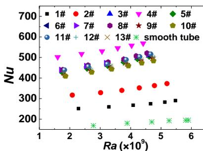
Figure 3: Variation of  $Nu$  with respect to  $Ra$  for the smooth tube, Vertical 3-D finned tubes
