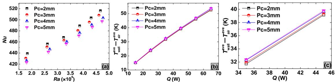
Figure 7: Effect of  $Pc$  on the air side heat transfer performance. (a)  $Nu$ , (b)  $T_{wall}^{ave} - T_{air}^{ave}$ , (c) Partial enlargement of b
