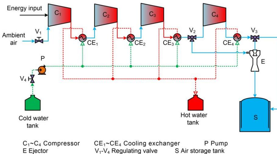
Figure 1: The diagram of charging process in EVA-CAES system
