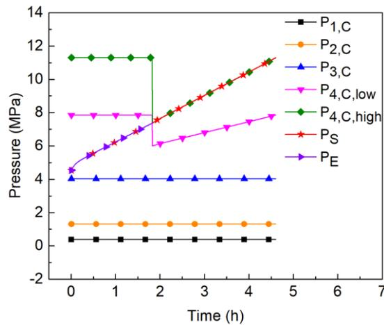
Figure 2: Variation of air pressure of compressors, ejector and air storage tank with time in EVA-CAES system
