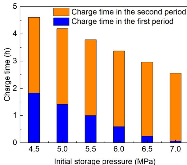
Figure 6: Variation of the charge time with initial storage pressure in EVA-CAES system.
