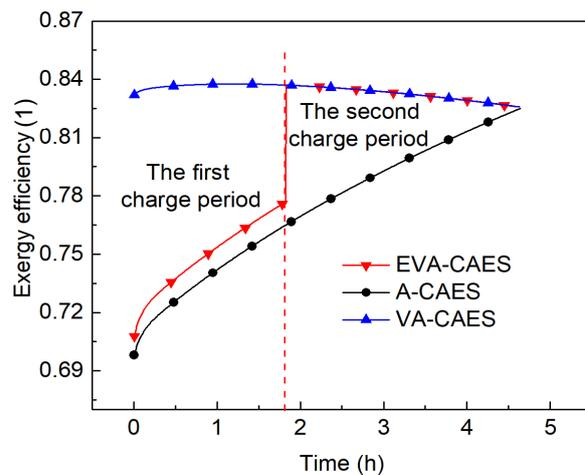
Figure 3: Variation of exergy efficiency with time
