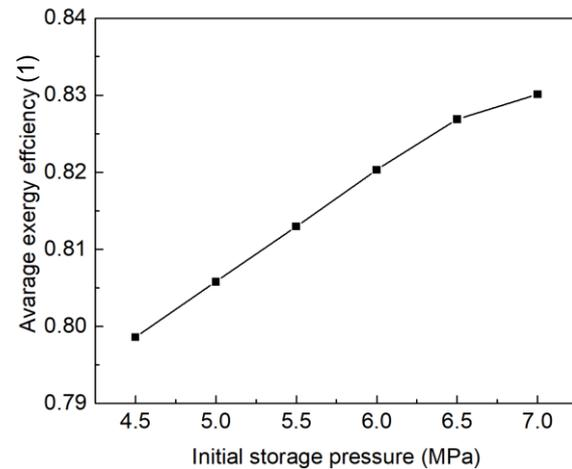
Figure 5: Variation of average exergy efficiency of EVA-CAES system with initial storage pressure
