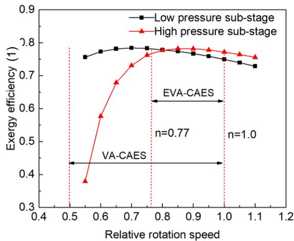
Figure 4: Variation of average exergy efficiency of EVA-CAES system with relative rotation speed
