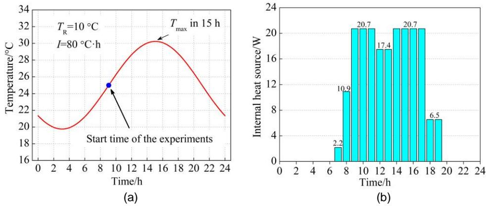
Figure 2: Experimental conditions: (a) outdoor air temperature; (b) power of indoor heat source
