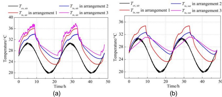
Figure 4: Temperature of the PCM wallboard with different material layer orders: (a) interior surface temperature; (b) indoor air temperature
