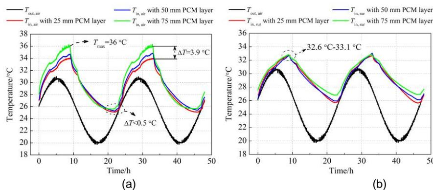
Figure 5: Temperature of the PCM wallboard with different PCM layer thicknesses: (a) interior surface temperature; (b) indoor air temperature
