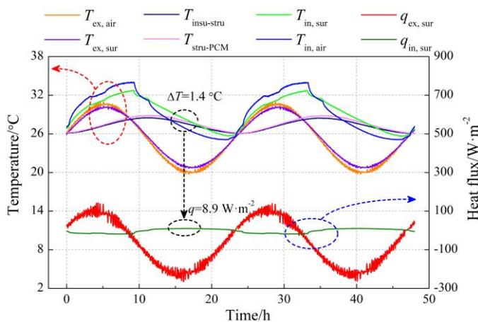
Figure 3: Temperature and heat flux of the PCM wallboard under double-sides periodic thermal effect
