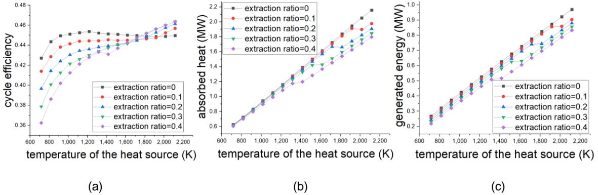
Figure 6: The change of the key parameters of the  $\text{SCO}_2$  Brayton recompression cycle under different extraction ratios with the temperature of the heat source: (a) Change in cycle efficiency; (b) Change in heat absorption; (c) Change in generated energy.
