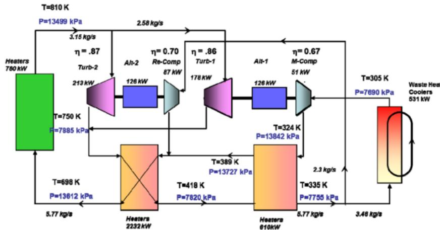
Figure 2: Schematic diagram of the Sandia recompression Brayton cycle experiment.
