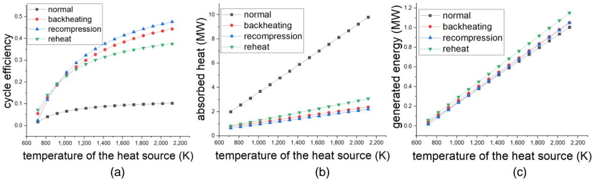
Figure 7: The variation of important cycle parameters of nitrogen Brayton cycle under four different models:(a) Change in cycle efficiency; (b) Change in heat absorption; (c) Change in generated energy.
