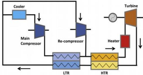
Figure 1: Typical layout of recompression Brayton cycle.
