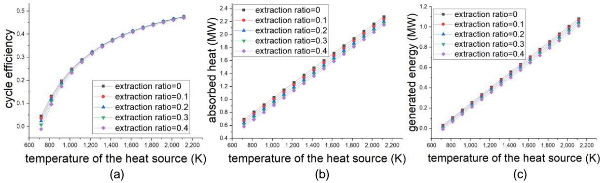
Figure 8: The change of the key parameters of the nitrogen Brayton recompression cycle under different extraction ratios with the temperature of the heat source: (a) Change in cycle efficiency; (b) Change in heat absorption; (c) Change in generated energy.
