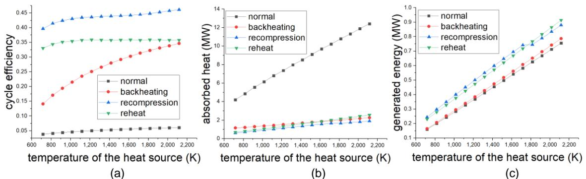
Figure 5: The variation of important cycle parameters of SCO<sub>2</sub> Brayton cycle under four different models: (a) Change in cycle efficiency; (b) Change in heat absorption; (c) Change in generated energy.
