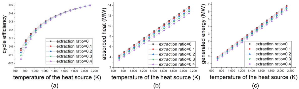
Figure 4: The change of the key parameters of the helium Brayton recompression cycle under different extraction ratios with the temperature of the heat source: (a) Change in cycle efficiency; (b) Change in heat absorption; (c) Change in generated energy.
