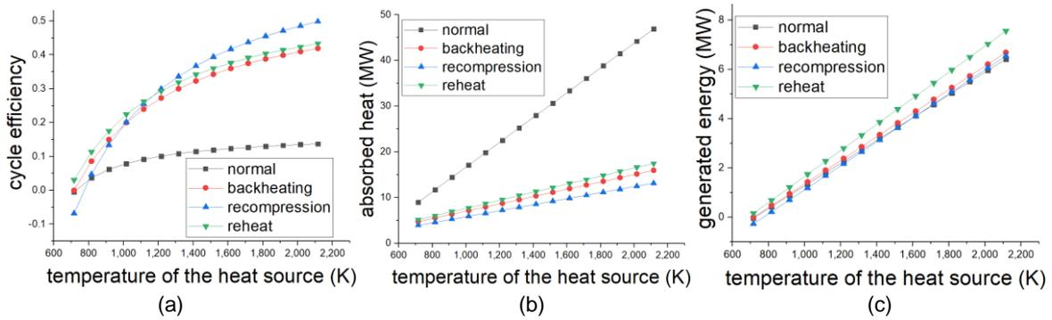
Figure 3: The variation of important cycle parameters of helium Brayton cycle under four different models: (a) Change in cycle efficiency; (b) Change in heat absorption; (c) Change in generated energy.
