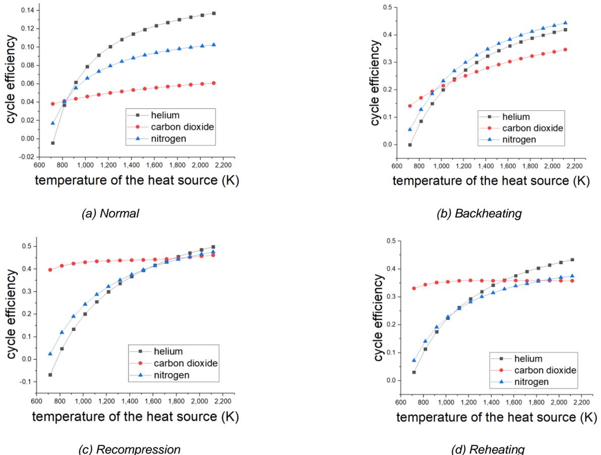
Figure 9: Comparison of working media under different Brayton cycle models
