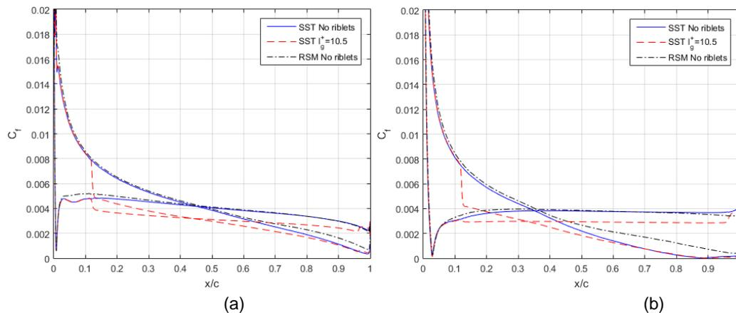
Figure 6: Comparison the computed skin friction coefficient with and without optimal riblets around the NACA airfoil at (a) 6 deg and (b) 12 deg angles of attack
