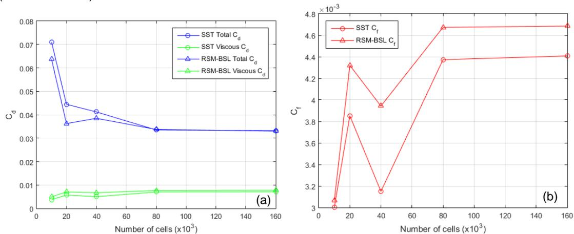
Figure 2: Variation of the (a) total and viscous drag and (b) friction coefficients with the computational grid size
