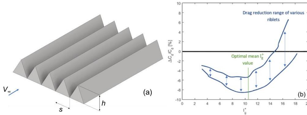
Figure 1: (a) V-groove riblet basic dimensions (b) Drag reduction as a function of the square root of groove cross section  $l_g^+$  for various types of riblets
