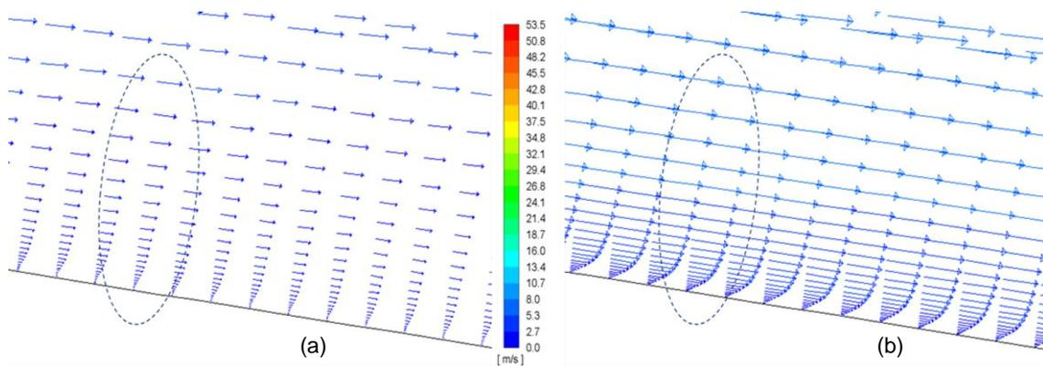
Figure 5: Velocity magnitude at the NACA 0012 trailing edge area at 10 deg angle of attack, using (a) the  $k-\omega$  SST and (b) BSL-RSM turbulence models.
