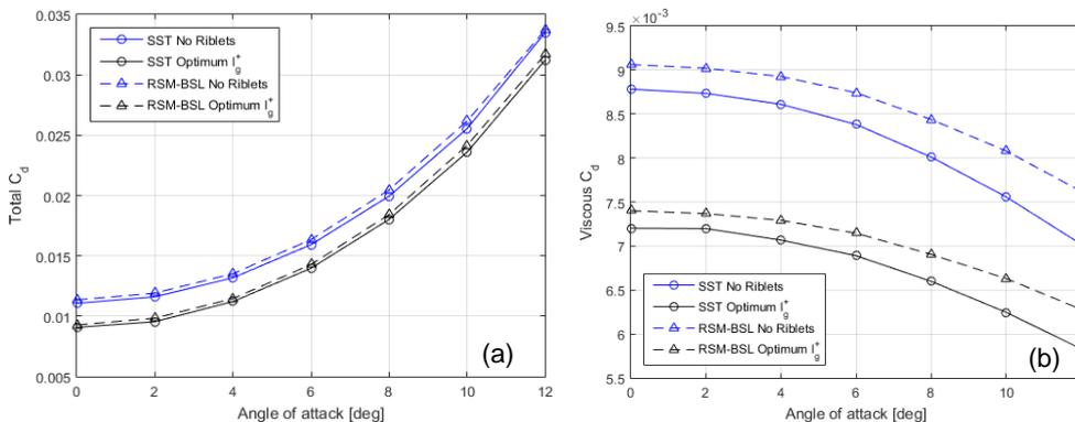
Figure 4: Comparison of (a) total and (b) viscous drag coefficients for a NACA 0012 airfoil with and without optimal riblet sizing ( $l_g^+=10.5$ ) for two turbulence models
