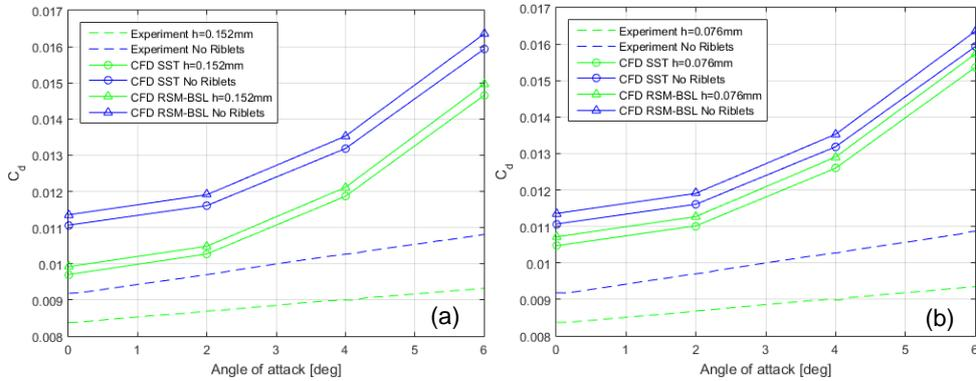
Figure 3: Comparison of  $C_d$  reduction between CFD results and experimental data (Sundaram et al., 1996) for riblet height (a)  $h=0.152$ mm and (b)  $h=0.076$ mm
