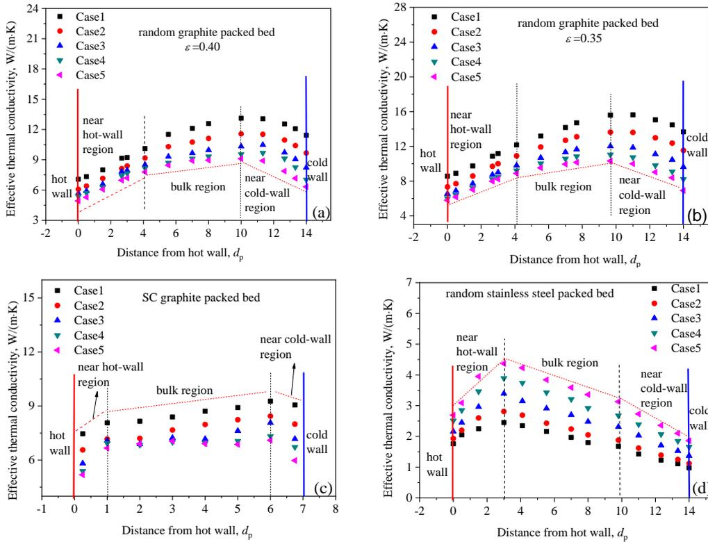
Figure 3: Effective thermal conductivity distributions in four different packed beds
