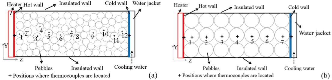
Figure 2: Schematic representation of a vertical section of test sections: (a) random graphite packed bed and (b) SC graphite packed bed
