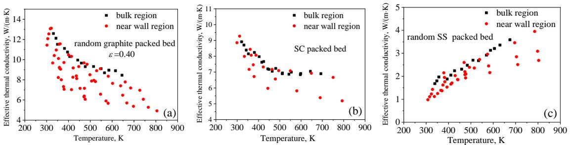
Figure 4: Effective thermal conductivity in near wall regions varying with temperature: (a) graphite packed beds ( $\epsilon=0.40$ ); (b) sc packed beds; (c) stainless steel packed beds
