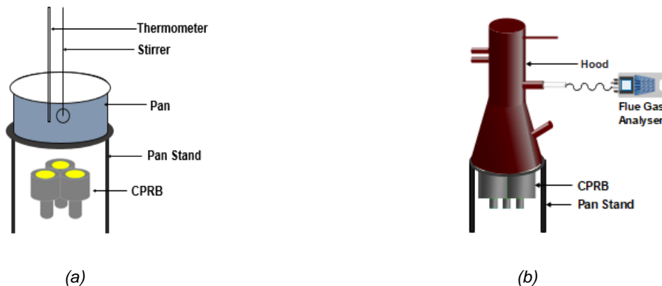
Figure 4: Schematic diagram for the measurement of thermal efficiency and emissions (a) Schematic diagram of the arrangement to measure the thermal efficiency (b) Schematic diagram of the arrangement to measure the emissions
