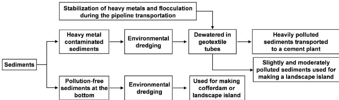
Figure 4: The flow diagram of sediments treatment
