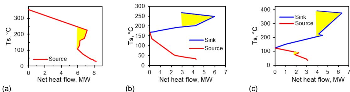
Figure 3: The GCC of three different hydrogenation processes for (a) Unit A; (b) Unit B; (c) Unit C
