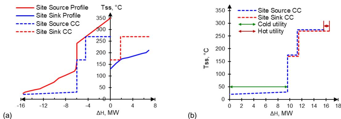
Figure 4: The Total Site Composite Curves (TSCC) (a) Total Site Profiles with utilities; (b) Hot Utility Generation Composite Curve (HUGCC)
