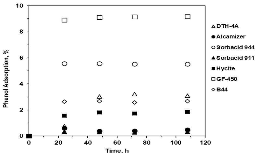
Figure 2: Phenol adsorption efficiencies of the various clays.
