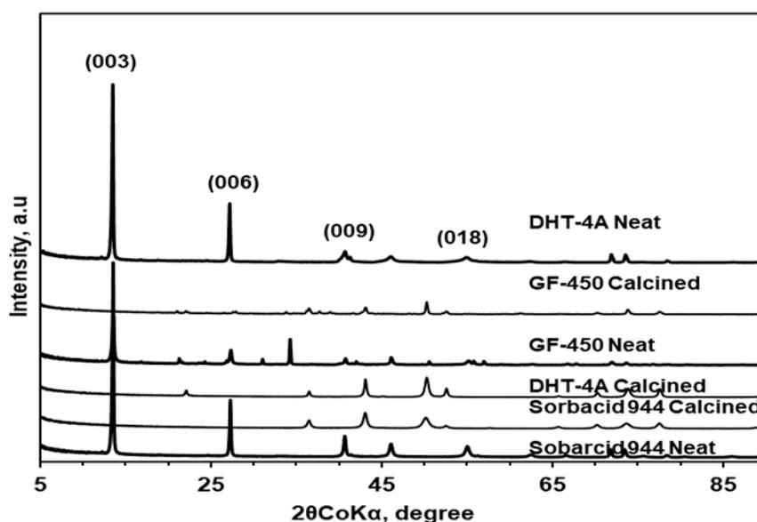
Figure 1: X-ray diffraction spectra of the neat and calcined clays.
