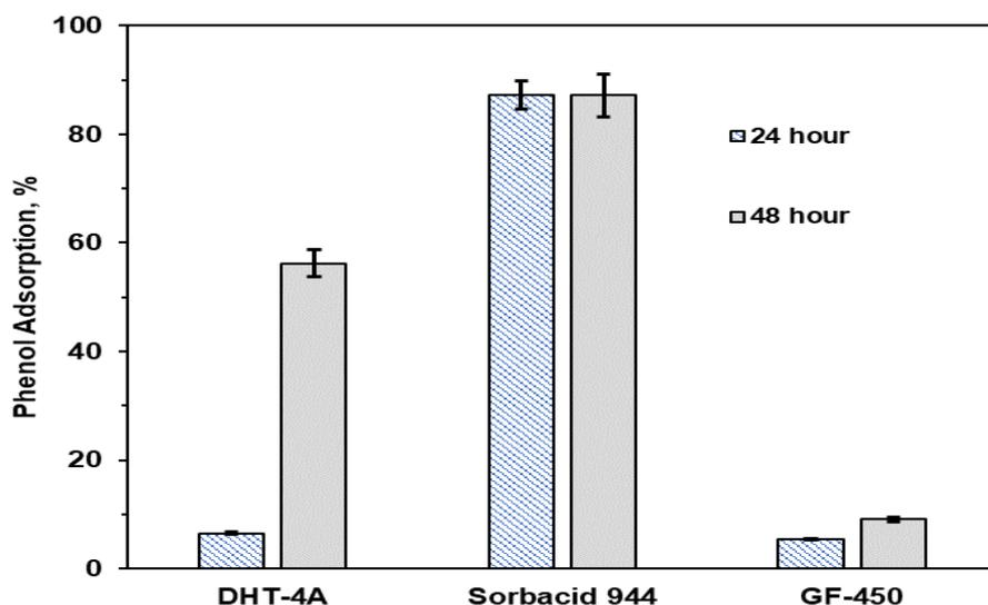
Figure 3: Phenol adsorption on calcined clays.
