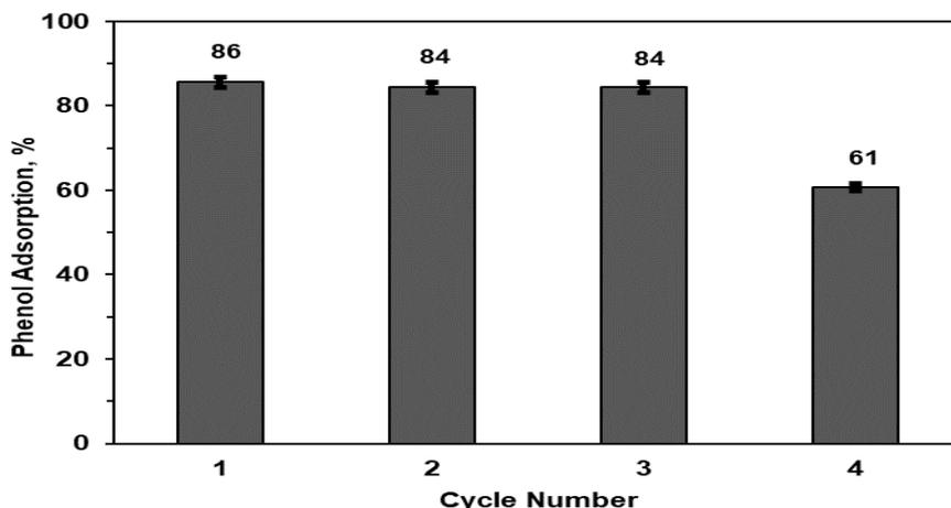
Figure 5. Phenol adsorption efficiencies on regenerated and re-used of clay.
