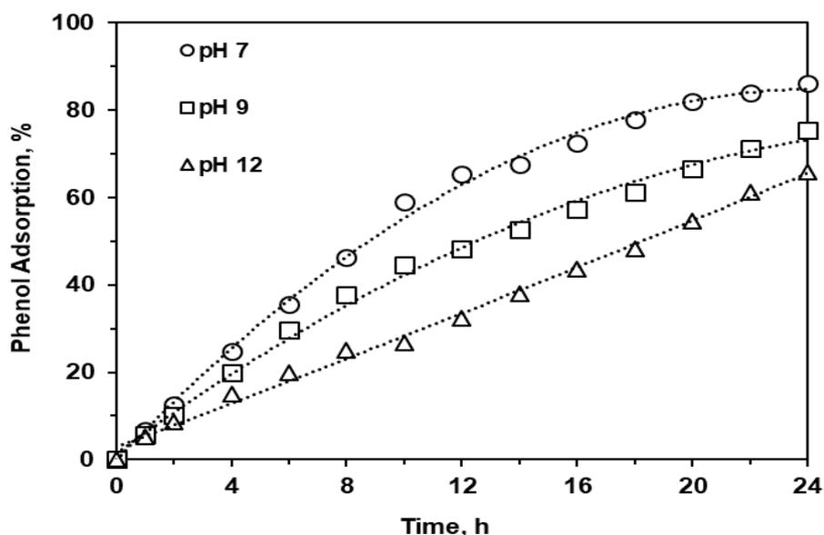
Figure 4: Effect of pH on phenol adsorption.
