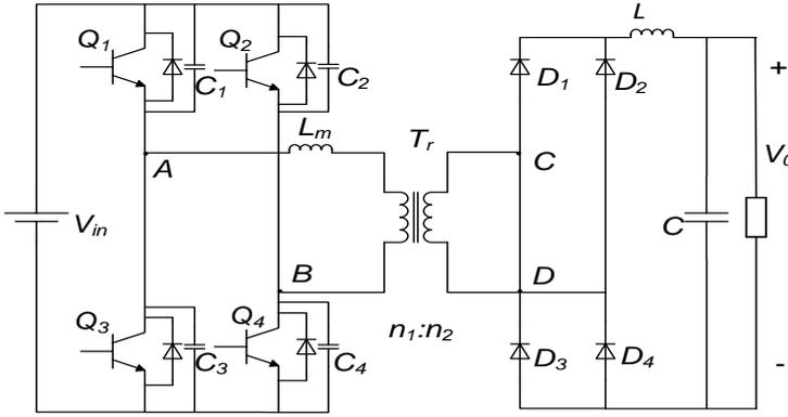
Figure 1: Isolated full-bridge DC-DC converter
