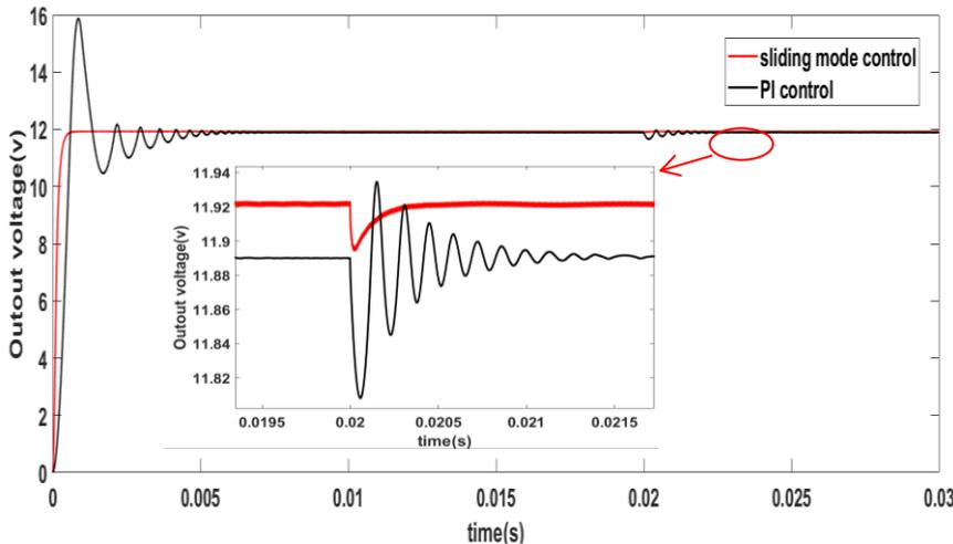
Figure 4: Output voltage when load resistance changed
