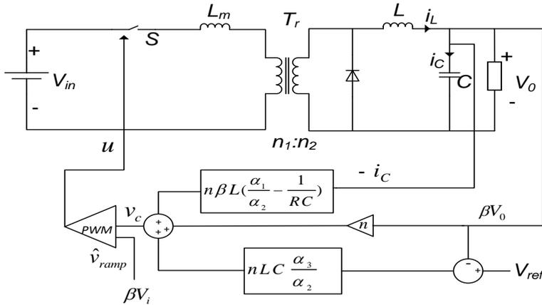
Figure 2: Block diagram of converter equivalent circuit and control structure of sliding mode converter
