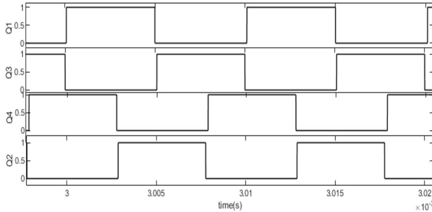
Figure 3: PWM drive signal waveform of the switch
