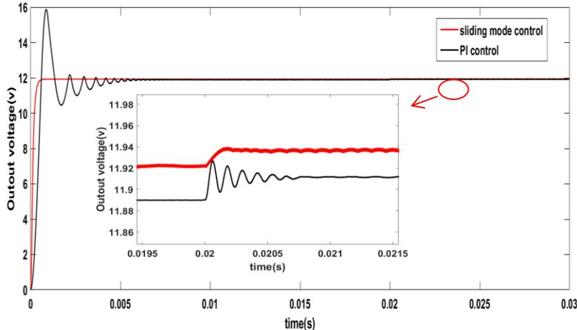
Figure 5: Output voltage when input voltage changed
