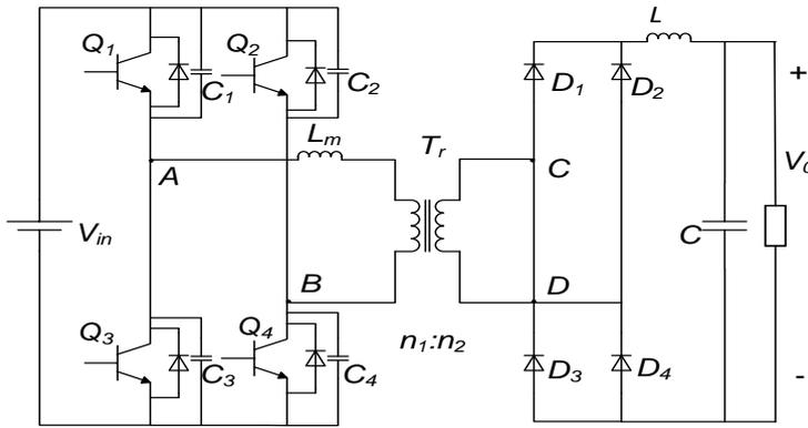
Figure 1: Isolated full-bridge DC-DC converter
