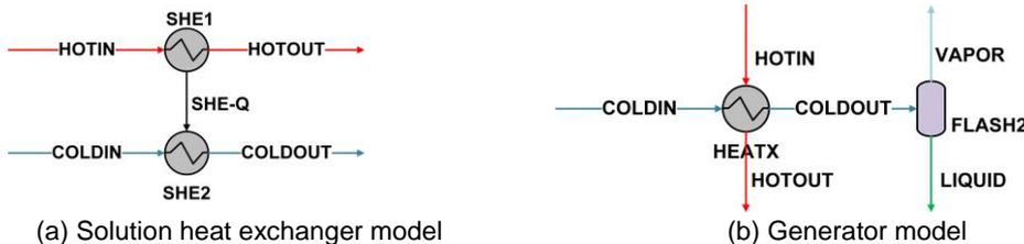
(a) Solution heat exchanger model
