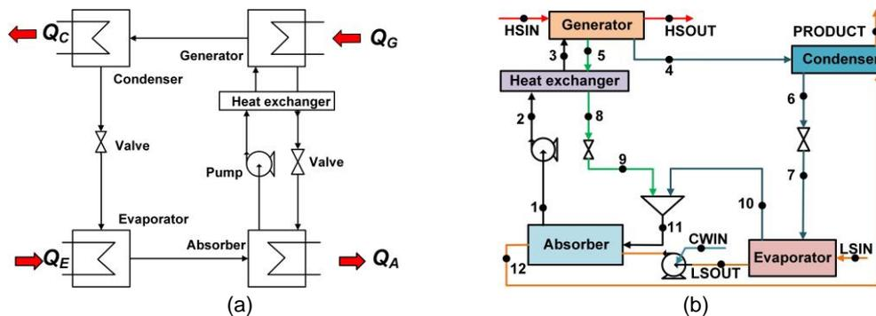
Figure 1: (a) Flowsheet of absorption heat pump / refrigeration cycle; (b) Selection of system state points
