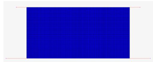
Figure 3: The mesh was made of around 600,000 tetrahedral elements.
