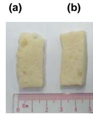
Figure 2: Salt leaching gelatin/CMC scaffold (a) G2.7T and (b) G2.4T, respectively.
