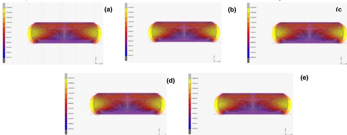
Figure 5: The finite element modeling of deformed salt leaching gelatin/CMC scaffold (a) G3T, (b) G2.7T, (c) G2.4T, (d) G2.1T and (e) G1.8T, respectively.
