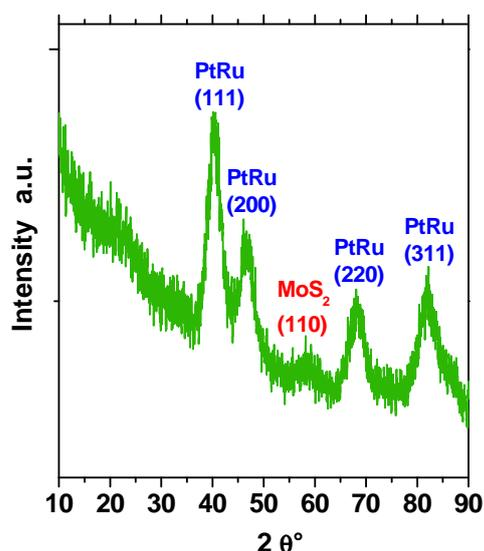
Figure 1: XRD spectrum of PtRu/MoS<sub>2</sub> NPs
