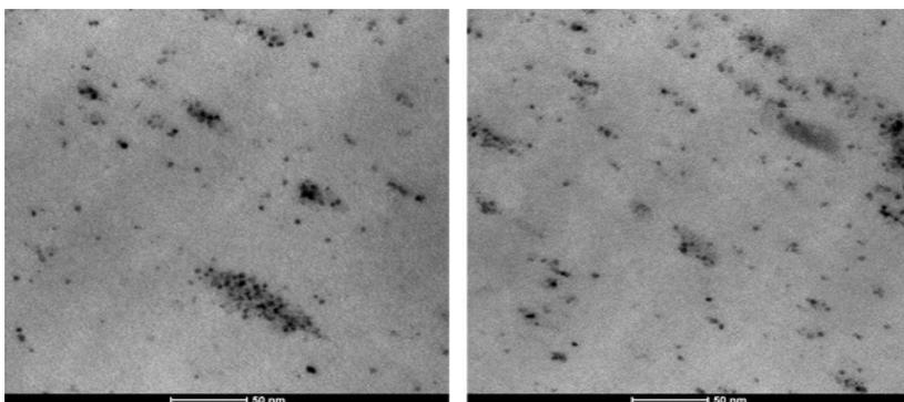
Figure 3: TEM image of dispersed of PtRu/MoS<sub>2</sub> NPs in HCL resin
