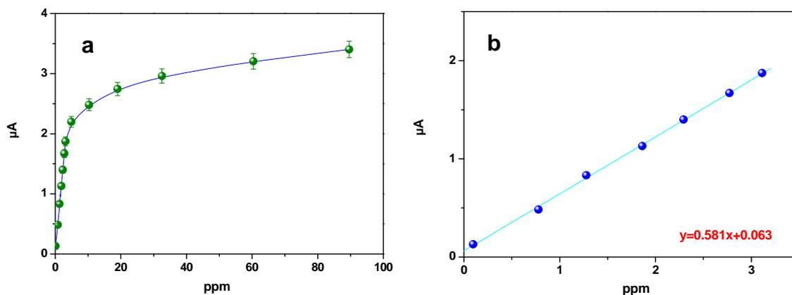
Figure 5: Amperometric sensitivity vs.  $\text{NH}_3$  concentration (a). Enlarged view of the first part of the curve and the fit of anodic peak current vs.  $\text{NH}_3$  concentration (b)
