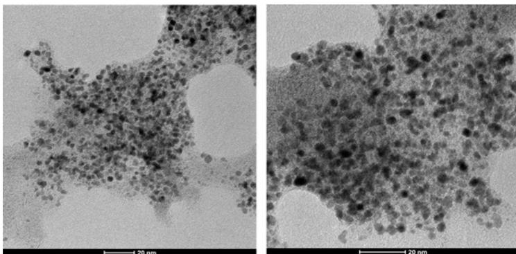
Figure 2: TEM images of PtRu/MoS<sub>2</sub> NPs at different magnifications
