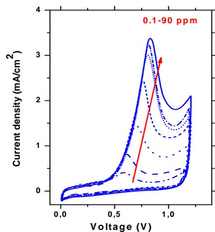
Figure 4: CV tests in the presence of different amounts of NH<sub>3</sub> in 1 M KOH
