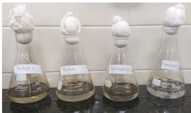
Figure 4: oil adsorbed to seawater by bioremediation process using the biosurfactant produced by C. sphaerica .
