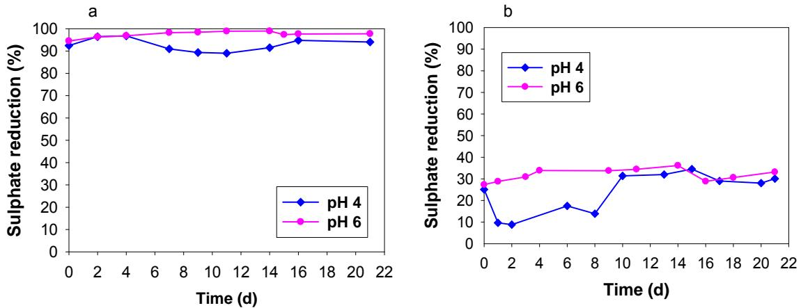
Figure 2: pH effect on sulphate reduction at (a) 20 °C and HRT of 7 d and (b) 10 °C and HRT of 4.5 d.
