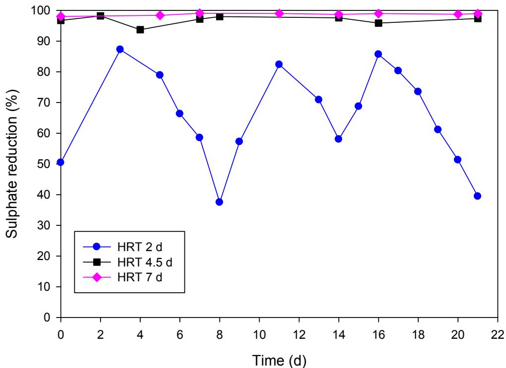
Figure 4: HRT effect on sulphate reduction at 30 °C and pH 5.
