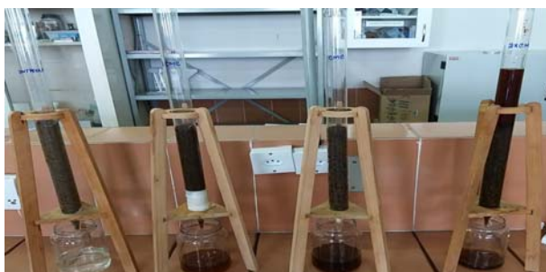
Figure 1: Glass columns used in the static test to remove engine oil impregnated in sand
