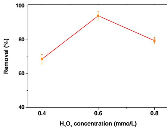
Figure 5. Effect of  $H_2O_2$  concentration on 2,4-dichlorophenol degradation. Immobilization conditions: coupling temperature, 4 °C; coupling pH, 6; lipase concentration, 0.1 mg/ml; time, 3 h. Degradation test conditions: reaction temperature, 25 °C; catalyst concentration 0.1 mg/ml; reaction time, 3h; 2,4-DCP concentration, 70 mg/L; pH, 6; Each point represents the mean of three experiments  $\pm$  S.E.
