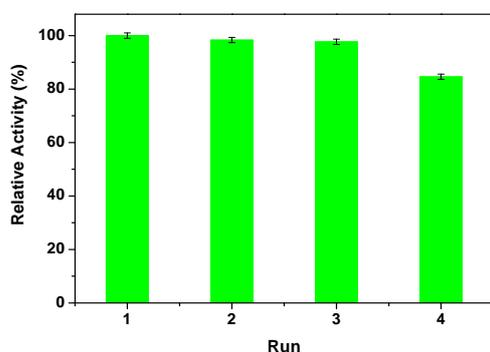
Figure 7. Recycling and catalytic stability of immobilized HRP. Immobilization conditions: coupling temperature, 4 °C; coupling pH, 6; lipase concentration, 0.1 mg/ml; time, 3 h. Degradation test conditions: reaction temperature, 25 °C; catalyst concentration 0.1 mg/ml;  $H_2O_2$  concentration, 0.6 mmol/L, 2,4-DCP concentration, 70 mg/L; pH, 6; reaction time, 3 h. Each point represents the mean of three experiments  $\pm$  S.E.
