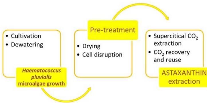
Figure 1. Natural astaxanthin production via *Haematococcus pluvialis* microalgae cultivation, dewatering, biomass drying and pretreatment, pigment extraction and carbon dioxide recovery and recycle.
