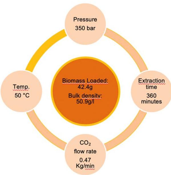
Figure 2. Optimized operational conditions adopted for extracting astaxanthin from *Haematococcus pluvialis* via supercritical CO<sub>2</sub> operation (Molino et al., 2018b, c).
