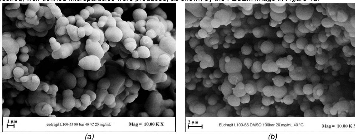
Figure 1: FESEM images of Eudragit particles precipitated from DMSO at 40 °C and 20 mg/mL. Effect of the operating pressure: (a) 90 bar; (b) 100 bar.
