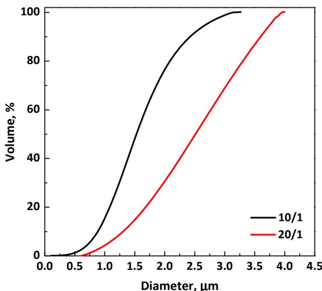
Figure 2: Volumetric cumulative PSDs of Eudragit/AMPI particles precipitated from DMSO at 40 °C, 100 bar, and 50 mg/mL; effect of the polymer/drug ratio.
