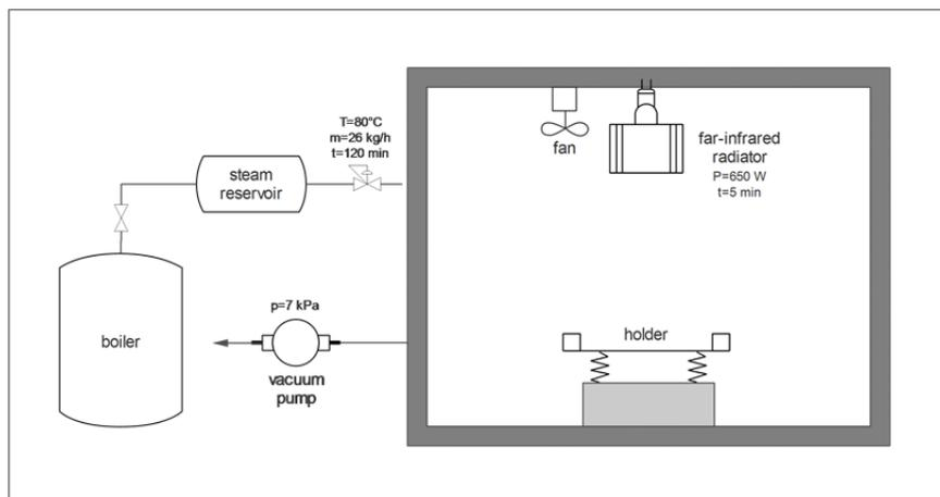
Figure 3: Flowsheet of the LPSSD-FIR process.
