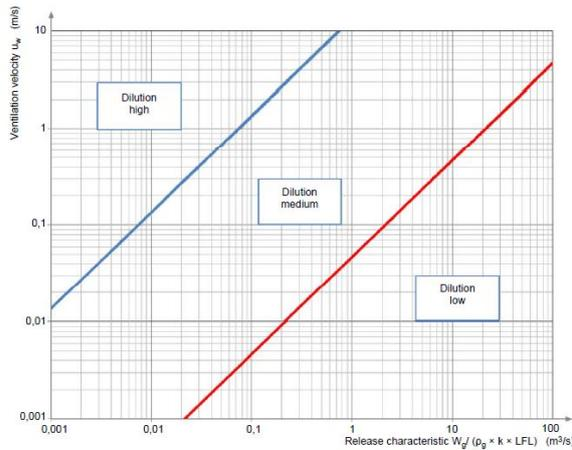
Figure 2: Dilution degree assessment (IEC EN 60079-10-1)
