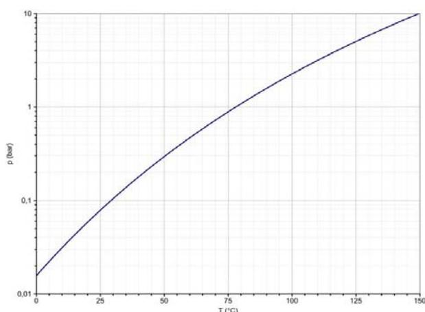
Figure 1: Bioethanol vapour pressure
