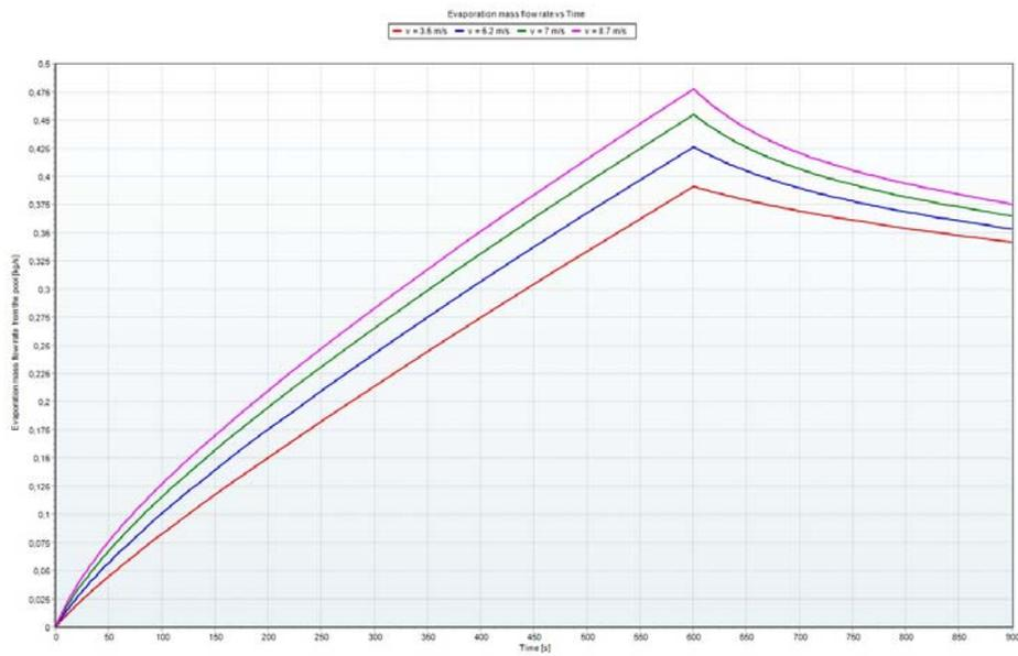
Figure 4: Trend of bioethanol evaporation rate
