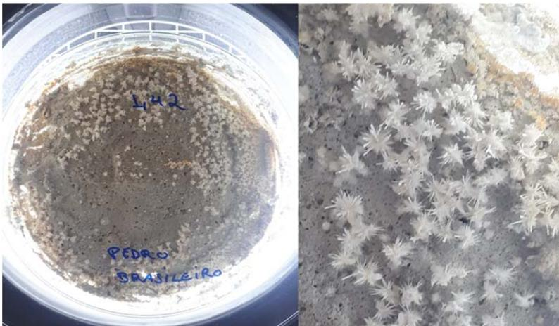
Figure 3: Crystal production after 168 h on the 1.42 g calcium lactate Petri Dish
