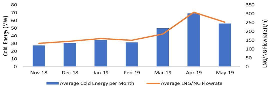
Figure 3: Graph of Average Cold Energy vs Send Out (NG Flow rate)
