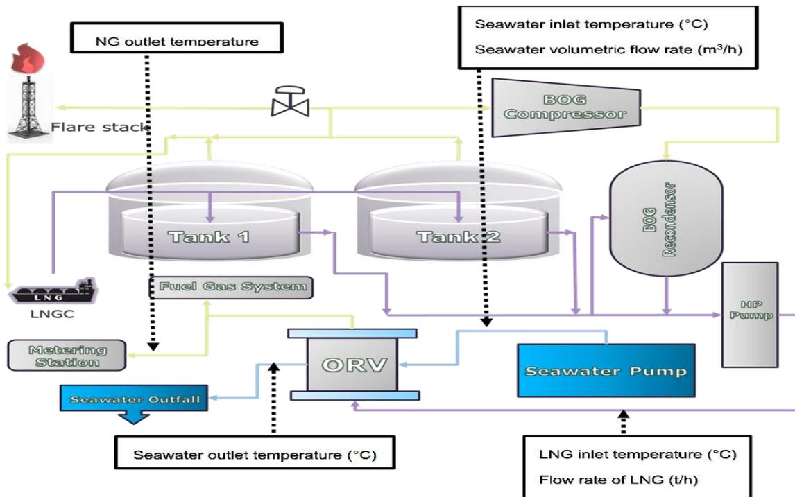
Figure 2: Process flow diagram of LNG regasification in PLNG2
