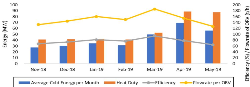
Figure 4: Graph of comparison of heat duty with average cold energy recovery
