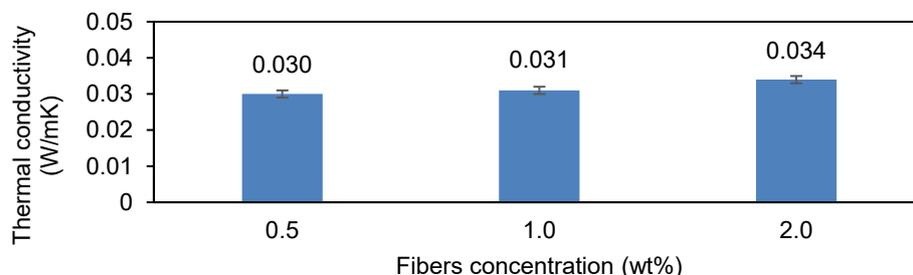
Figure 5: Thermal conductivities of the PFs aerogels with different PFs concentrations.
