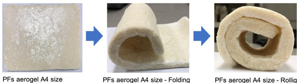
Figure 6: Good flexibility of developed PFs aerogels from the PFs.
