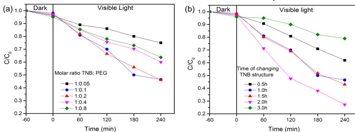
Figure 5: Photocatalytic degradation of phenol over  $TS05$  (a) Effect of molar ratio  $TNB:PEG$ ; (b) Effect of the time of heating  $TNB$  and  $ACAC$
