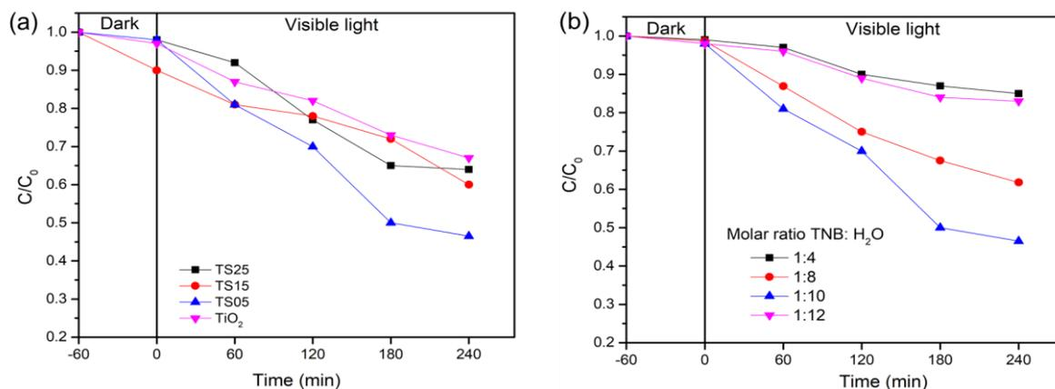
Figure 4: Photocatalytic degradation of phenol (a) Effect of molar ratio  $TiO_2:SiO_2$ ; (b) Effect of molar ratio  $TNB:H_2O$  over  $TS05$
