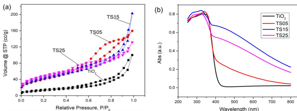
Figure 3: (a) N<sub>2</sub> adsorption–desorption isotherms; (b) The band-gap energy of TiO<sub>2</sub>, TiO<sub>2</sub>/SiO<sub>2</sub> samples
