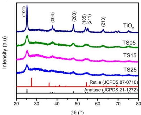
Figure 1: X-ray patterns of  $\text{TiO}_2$ , TS05, TS15 and TS25
