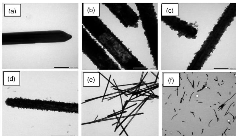
Figure 1: TEM images of: (a) AgNWs (scale bar 100 nm); (b) PdAg-MW6 (scale bar 100 nm); (c) PdAg-MW10 (scale bar 100 nm); (d) PdAg-CP (scale bar 200 nm); (e) PdAg-MW6 (scale bar 1  $\mu$ m); (f) PdAg-MW12 (scale bar 2  $\mu$ m).
