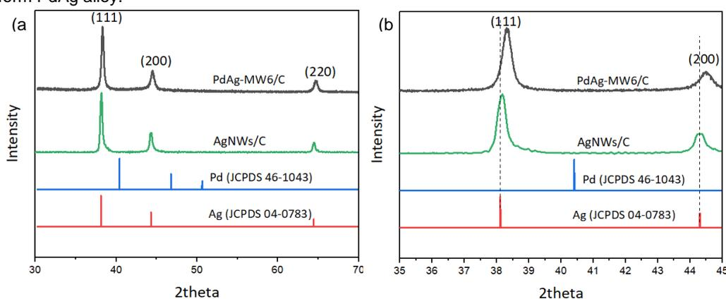
Figure 2: XRD patterns of AgNWs/C and PdAg-MW6/C:(a) from 30 to 70 ° and (b) from 35 to 45 °
