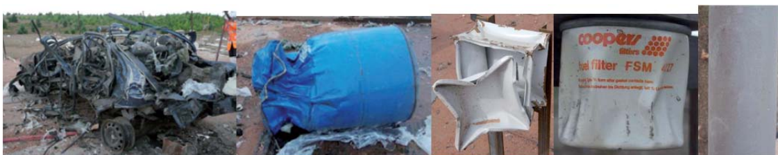
Figure 1: Damage to some of the items placed inside a propane detonation (Burgan, 2014). Damage created by overpressure > 10 bar. Note the dark markings on the post (extreme right) facing opposite to detonation propagation.
