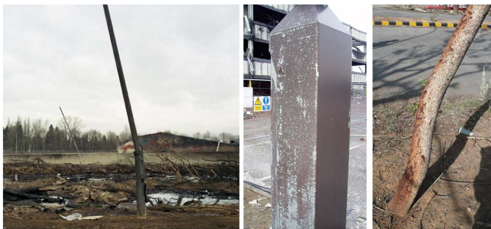
Figure 2: Examples of directional indicators from Buncefield (left and centre) and Jaipur
