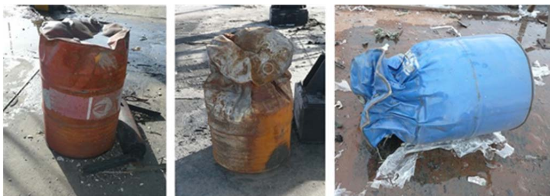
Figure 4: Recorded damage to oil drums at Jaipur (left and centre) and a drum from a detonation test (right)
