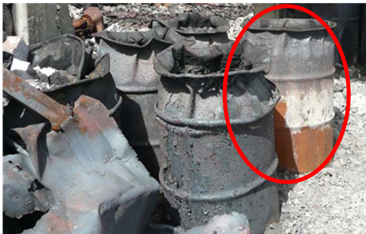
Figure 3: Damage to oil drums immediately adjacent to that shown in the HSE 2017a (circled)
