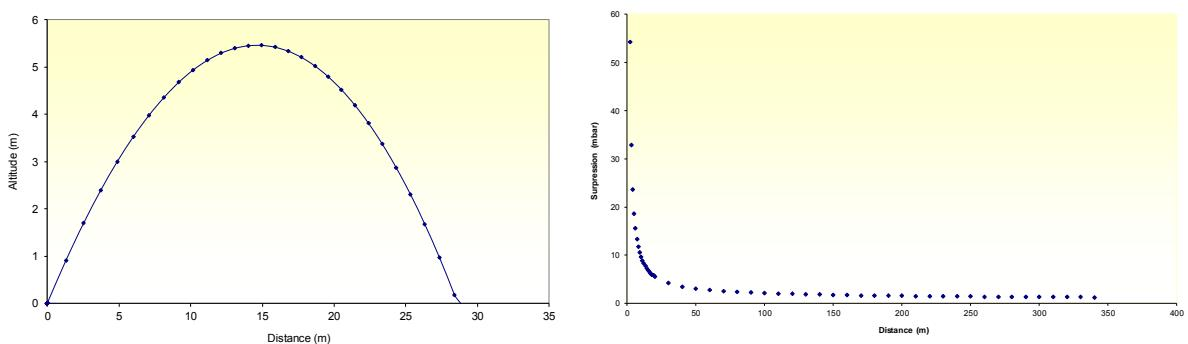
*Figure 1. Maximum projection distance (a) and overpressure (b) as a function of distance to the reactor calculated with PROJEX EPHEDRA software.*
