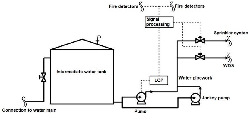
Figure 3: Reference scheme of firefighting water network. The system is connected to sprinklers and to WDS; LCP: local control panel.
