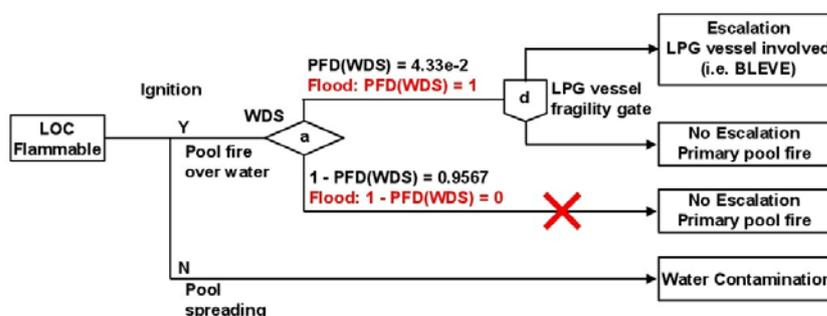
Figure 4: Event Tree for Natech-domino accident triggered by flood. PFD for LPG protection WDS is reported in black (Landucci et al., 2016), while tailored PFD for WDS in case of flood is in red. BLEVE: boiling liquid expanding vapour explosion. See (Landucci et al., 2016) for gates definition.
