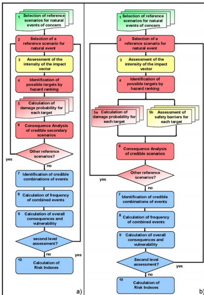
Figure 1: a) Procedure developed by Cozzani et al. (2014). b) Tailored procedure accounting for safety barriers. The barrier assessment is carried out in a dedicated parallel node (node 5b).
