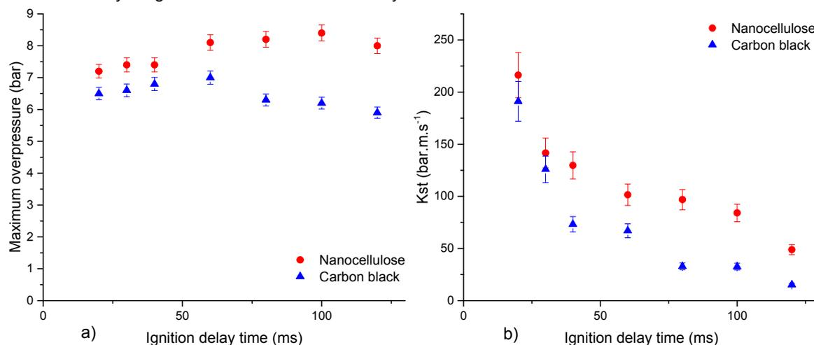
Figure 2: Evolution of (a-left) the maximum overpressure and (b-right) the deflagration index  $K_{St}$  of nanocellulose ( $750 g \cdot m^{-3}$ ) and carbon black ( $250 g \cdot m^{-3}$ ) as a function of the ignition delay time
