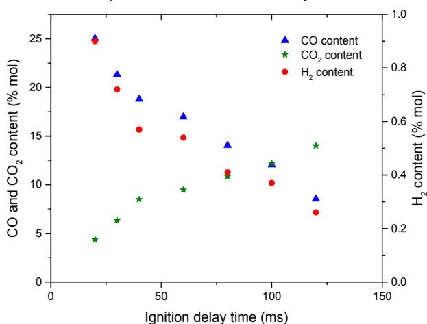
Figure 3: Evolution of the hydrogen, carbon monoxide and carbon dioxide content after combustion of carbon black nanopowders as a function of the ignition delay time
