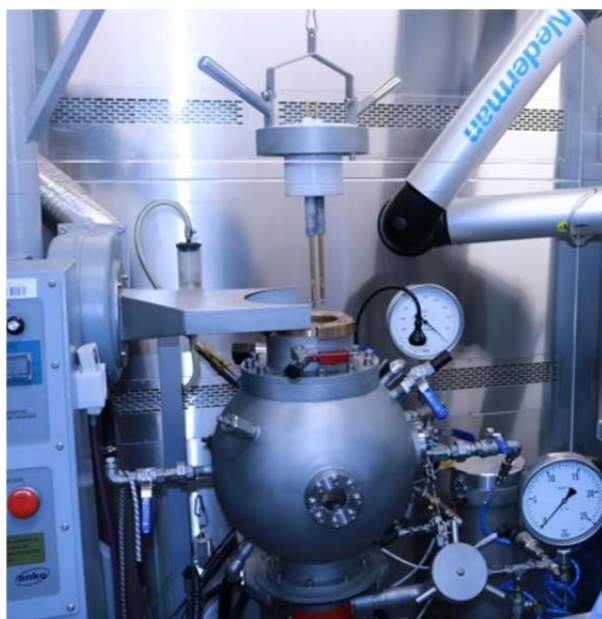
Figure 1: 20 litre sphere ANKO
