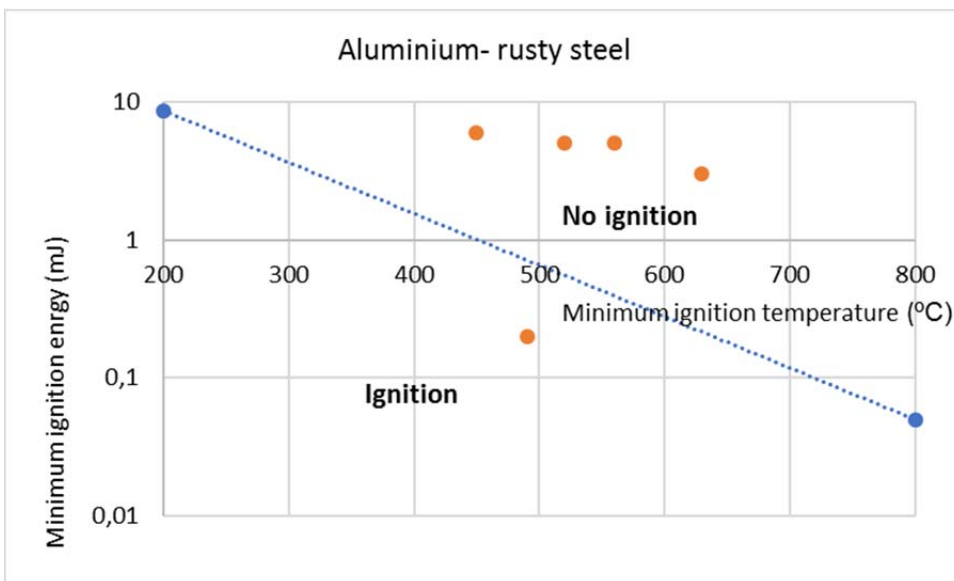
Figure 3: Relationship distinguishing between fuels that can be ignited by steel grinding sparks as suggested by Ritter (1984) compared to results by Schulz and Dittmar (1963).
