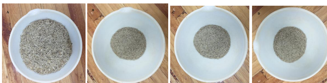
Figure 2: Photographs of the various particle sizes of the sugarcane bagasse for (A) 2.0 mm, (B) 1.0 mm, (C) 0.6 mm and (D) 0.4 mm
