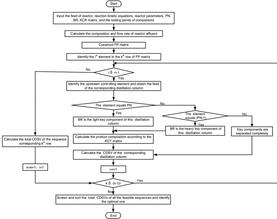
Figure 4: Procedure for identifying the optimal distillation of RDR system
