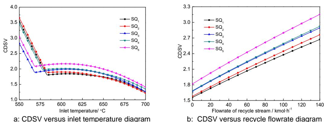
Figure 5: The total CDSVs of five distillation sequences at different inlet temperature and recycle flowrate
