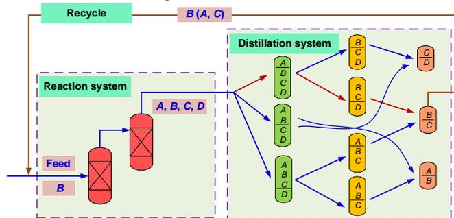
Figure 1: Simplified flow chart of 4-component RDR system
