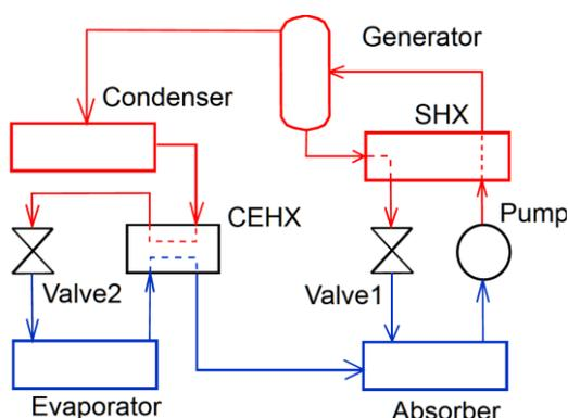
Figure 1: Single-stage, single-effect  $\text{NH}_3/\text{H}_2\text{O}$  ABR configuration.
