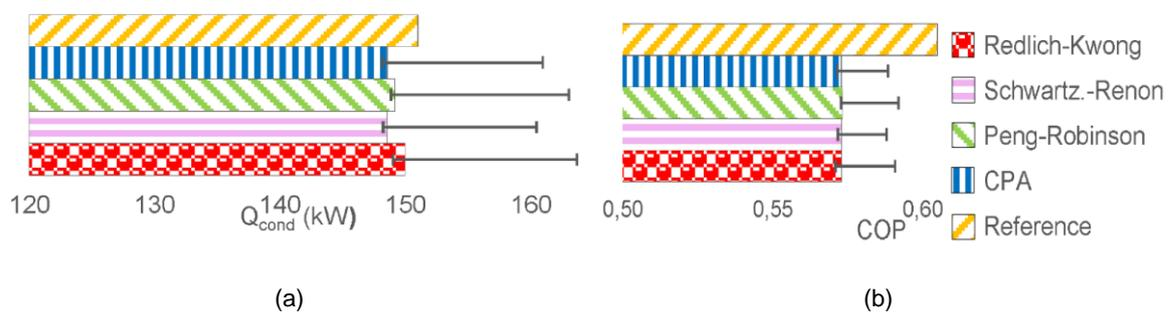
Figure 3: (a) nominal  $Q_{cond}$  and (b)  $COP$  values under variability (black errorbars) compared to reference values (Adewusi and Zubair, 2004) on ABR single-effect process.
