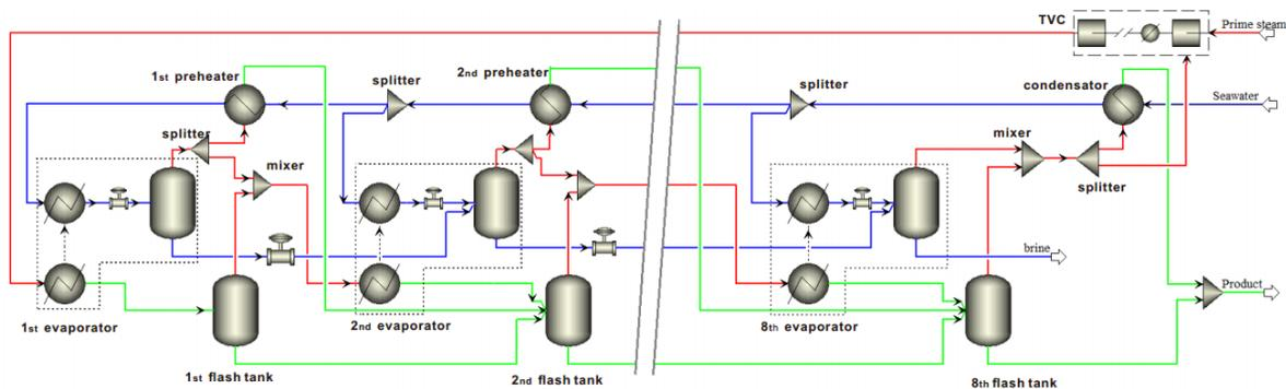
Figure 2: Aspen model of the eight-effect MED-TVC system
