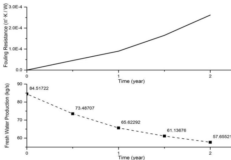
Figure 4: Variation curves of the first-effect evaporator fouling thermal resistance and optimal fresh water production
