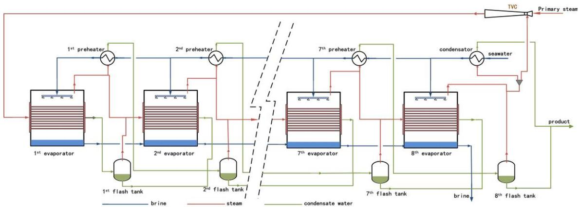
Figure 1: The construction of the eight-effect MED-TVC dynamic model
