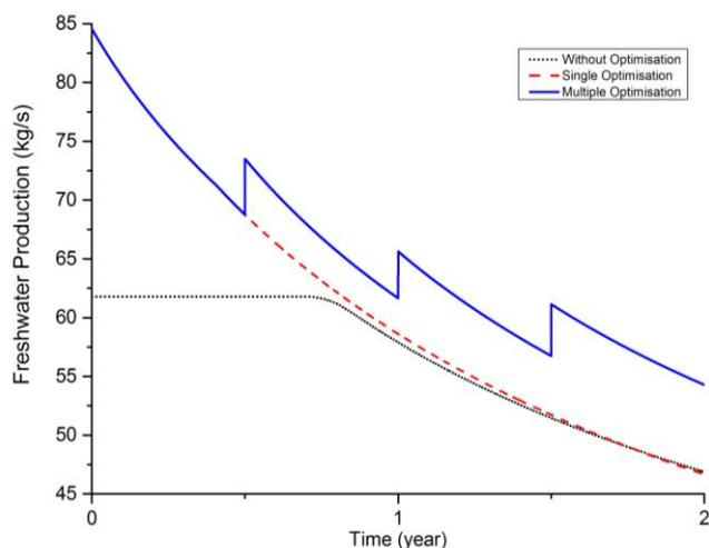
Figure 5: Fresh water production with single optimisation, multiple optimisation and without optimisation
