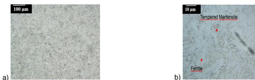
Figure 1: a) Micrographs of ASTM A335 P92 steel before exposure to corrosive environments, 100 µm; 1b) Micrographs of ASTM A335 P92 steel before exposure to corrosive environments, 10 µm
