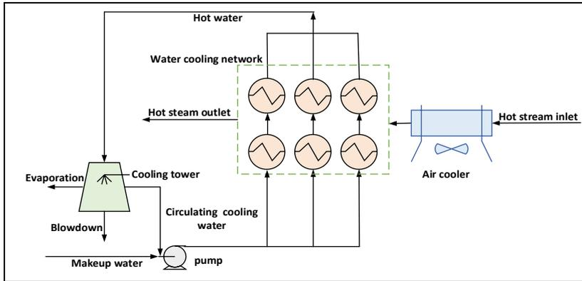
Figure 1: The structure of cooling water system with air coolers
