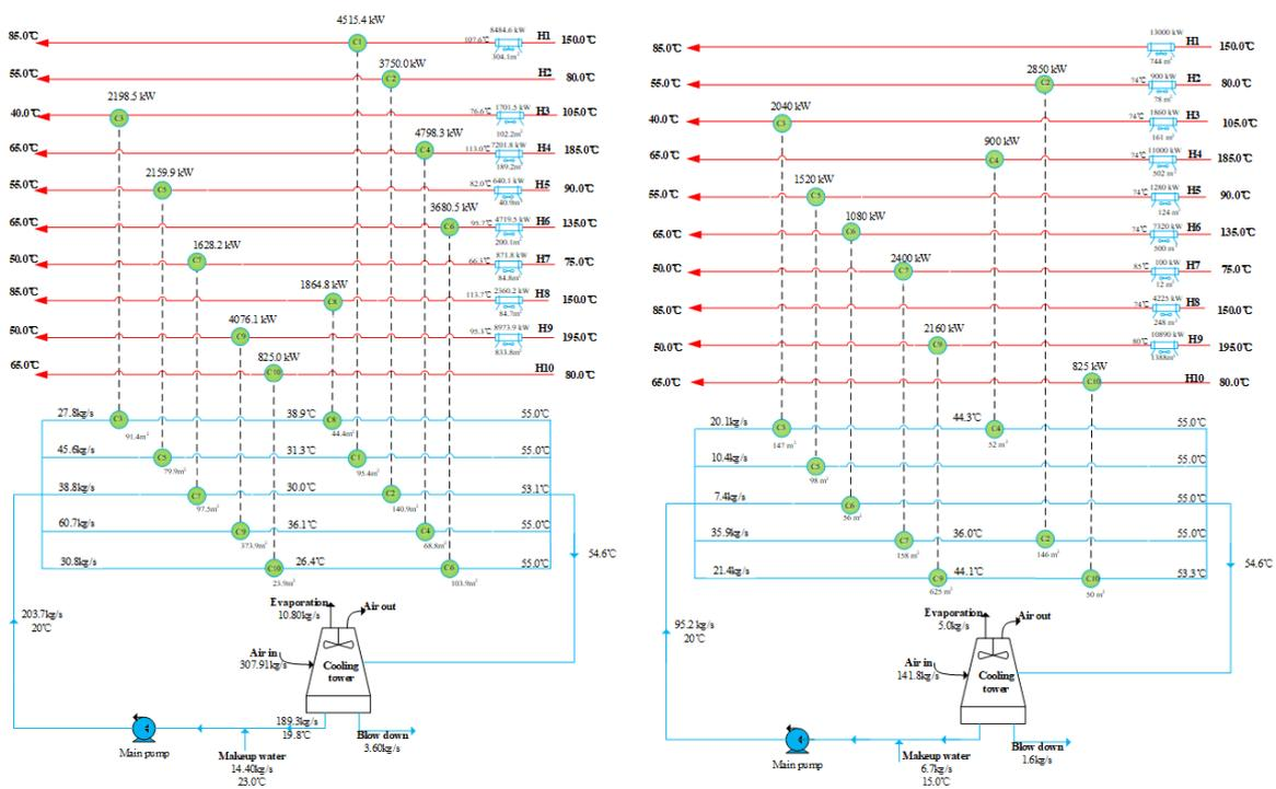
Figure 3: The network of case study (left: original network, right: optimal network)
