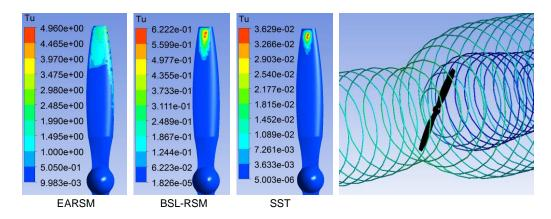
Figure 7: Tu distributions (left) and flow streamlines for the rotating reference frame (right)
