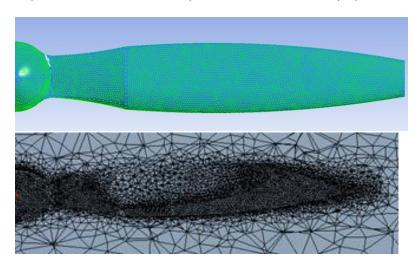
Figure 2: Representative views of the computational mesh around the propeller
