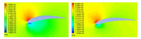
Figure 5: Pressure contours for stations 2(left) and 3(right)
