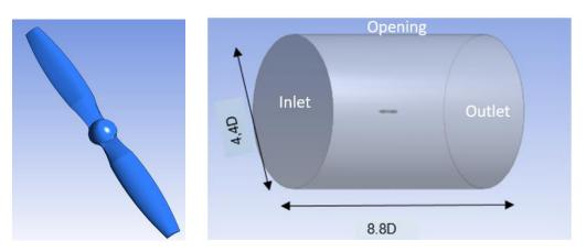
Figure 1: Indicative view of the propeller geometry and the computational domain
