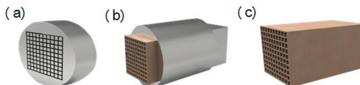
Figure 1: Modeling an extrusion process for the production of block ceramics (a) a matrix, (b) an extrusion process, (c) catalyst block carrier
