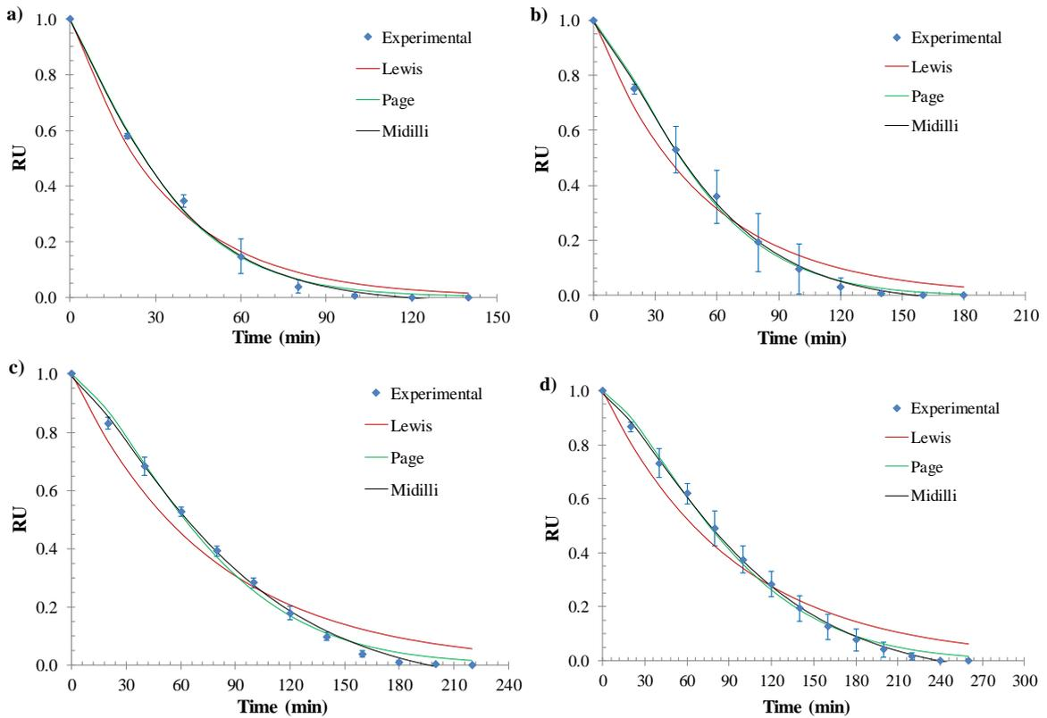
Figure 1: Comparison between the models used for green acerola in thicknesses (a) 3 mm, (b) 4 mm, (c) 5 mm and (d) 6 mm
