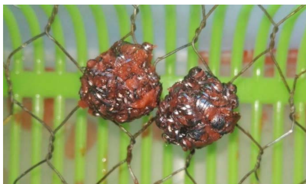
Figure 2. Soiled substrate with mixed fat-starch soil (80% w/w fat – 20% w/w starch)
